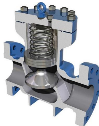
API Spec 6D Figure B.13—Piston Check Valve
