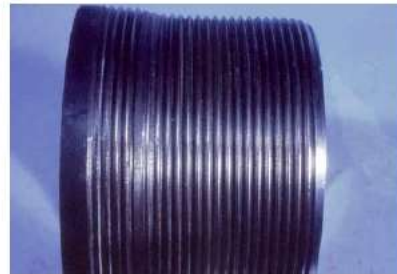
NOTE Improper taper.
