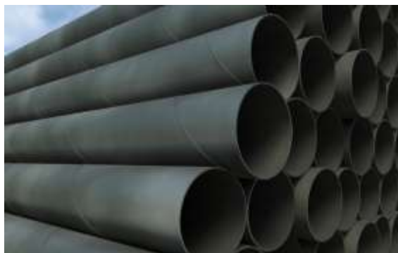
Helical (Spiral) seam
