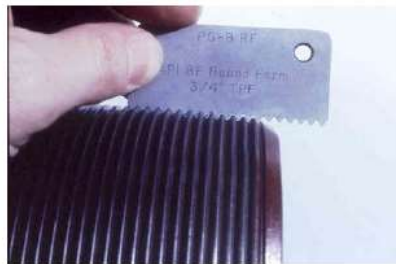
NOTE Profile gauge highlights improper thread form.
