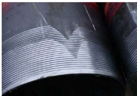
NOTE Effect of a flat spot. Figure 120
