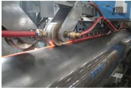
Electric Resistance Welded- ERW
