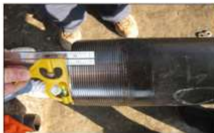
NOTE Scale shows length of perfect thread. Figure 119
