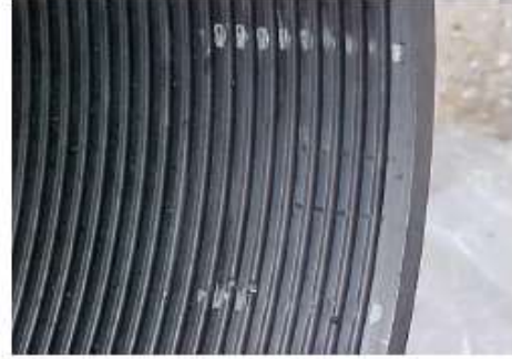
NOTE Internal coupling threads. Figure 142
