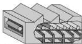
Shell Reheated in a Furnace.
